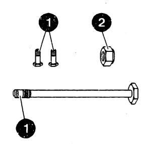
The following components are required for pinion attachment on starters up to FD 821 (Jan. 78):
